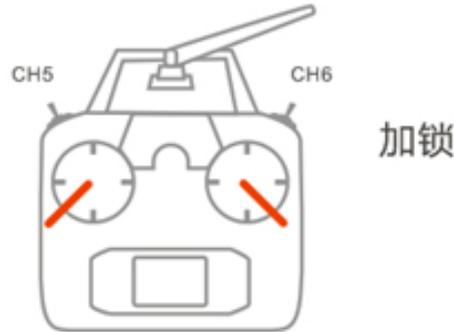
**Note:** Do not pull the stick as is shown in the above figure during flight, otherwise the motor will stop spinning immediately.
