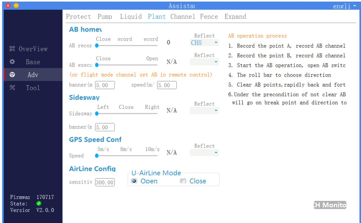
**3、Operation:** switch to “Close”—“Move to the left”—“Close”, and it will execute a left side-move once; switch to “Close”—“Move to the right”—“Close”, and it will execute a right side-move once.
