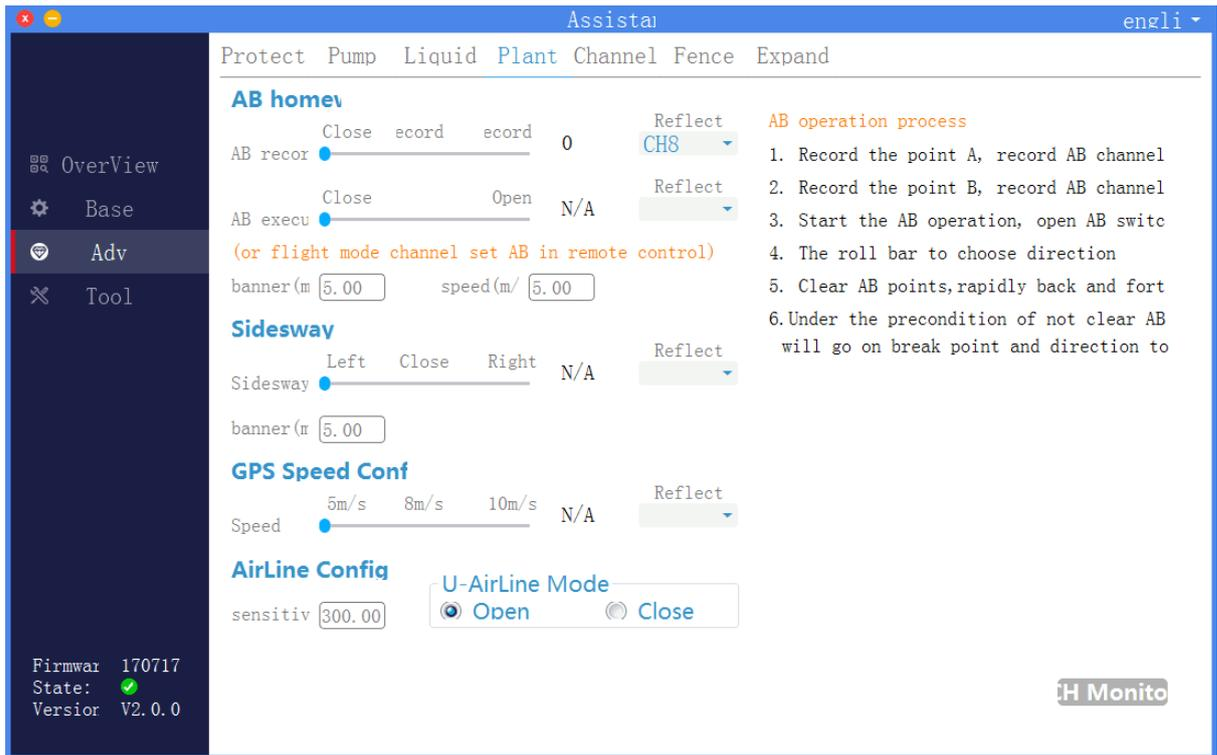
**2、 Operation:**the maximum flight speed can be limited at 5m/s,8m/s or 10m/s by switching the control stick when the aircraft is flying under GPS speed mode.
